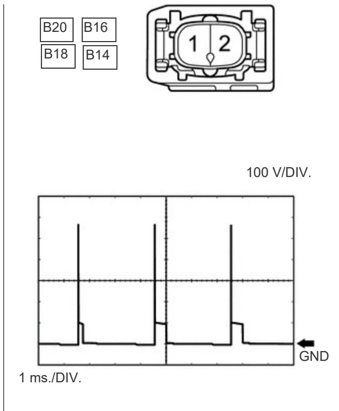
\*a Front view of wire harness connector (to Injector Assembly)
