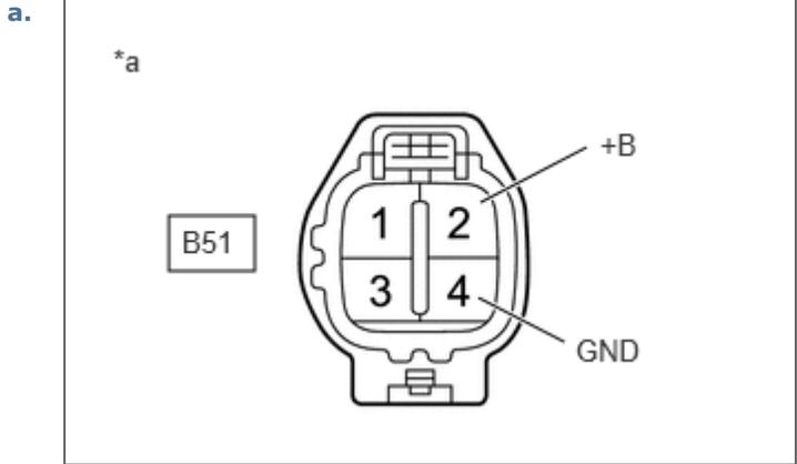
\*a Front view of wire harness connector (to Injector Driver (EDU))
